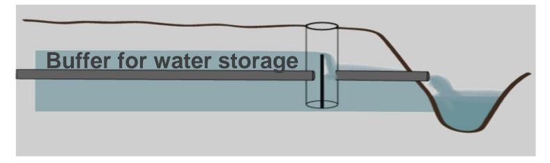
Controlled drainage can level out the inflow of drainage water to a constructed wetland
